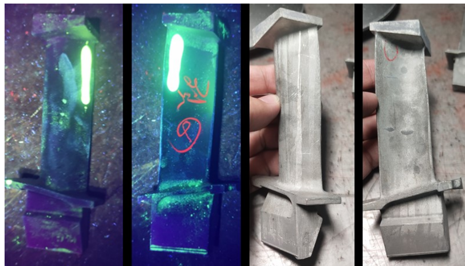
Figure 7. The fluorescence detection and macroscopic grain corrosion of the hot cracked blade, and the red circle is the hot crack.
