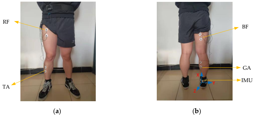
Figure 2. Electrode attachment point and IMU position. (a) Frontal side of human lower limbs; (b) back side of human lower limbs.
