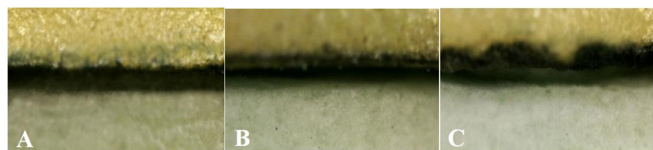
Figure 9. Marginal fit of PFM dental restoration after final glazing procedure at \times 300 magnification (A) casting, (B) milling, (C) SLM.
