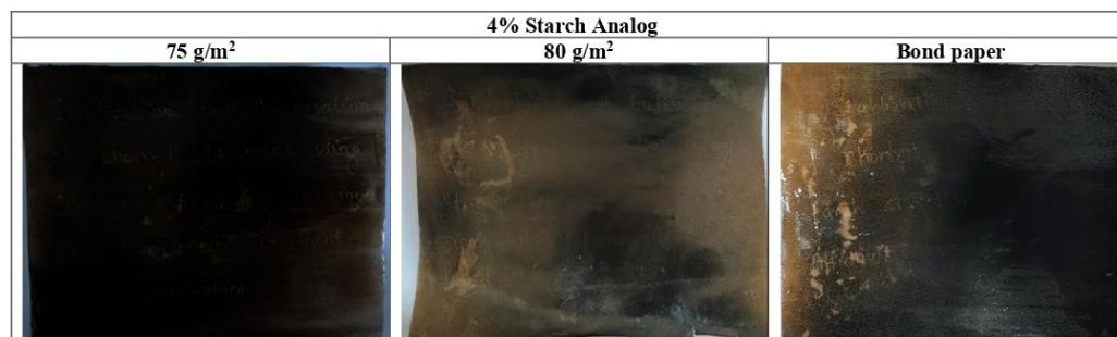
**Figure 6.** Coated and preserved charred samples with 4% starch analog on 75 g/m<sup>2</sup>, 80 g/m<sup>2</sup>, and bond paper (affidavit) written with Linc Pentonic blue ballpoint pen.
