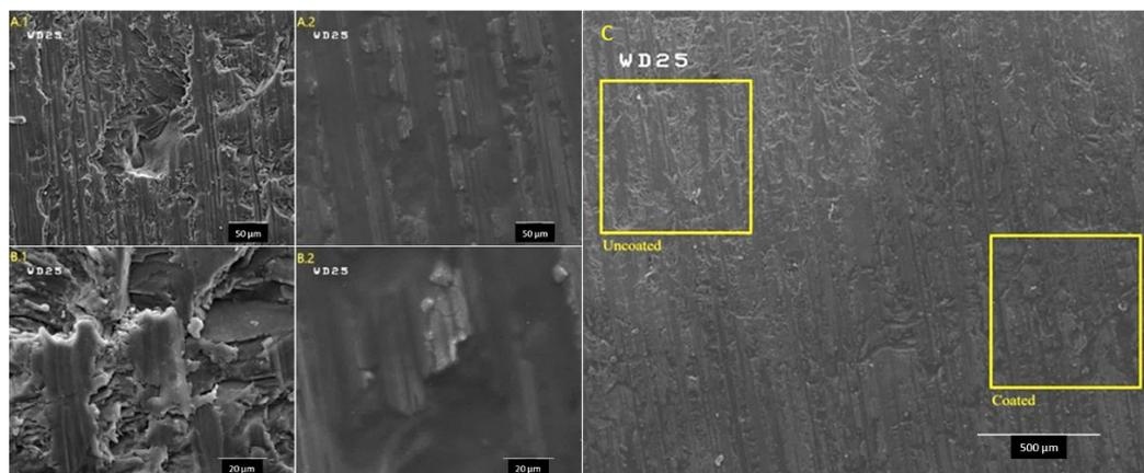
**Figure 2.** SEM images at 300 $\times$  (A) and 1000 $\times$  (B) magnifications comparing the bare (1) and coated (2) surfaces of a marble sample, primarily calcite, treated with formula 11. SEM image (C) of the transitional region between surfaces at 50 $\times$  magnification, the darker region has been coated.
