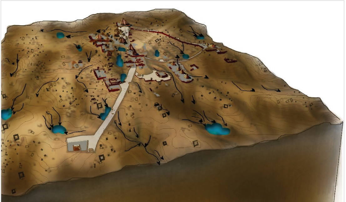
Figure 9. Water management in Tikal: The image shows the flow of water under gravity from the watershed created on the hill's summit. The water is then stored in the low-lying bajos (natural and human-made water reservoirs) that dot the landscape for use by the common people especially during the dry season. This shows an increased understanding by the Maya of their climate and terrain (adapted from Lucero & Gonzalez Cruz [48] (p. 6)).
