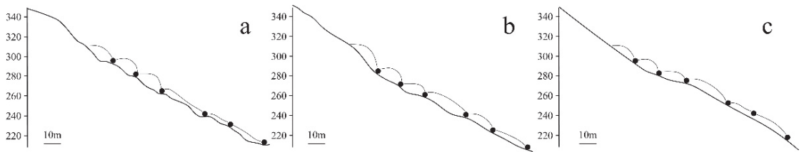
Figure 12. Theoretical 2D profiles of a rockfall event, drawn on a topographic profile extracted from the 1 m resolution DEM (a), the 5 m resolution DEM (b) and the 30 m resolution DEM (c).
