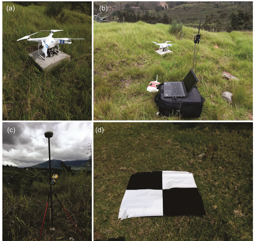
Figure 3. (a) Phantom 2 equipped with a ventral camera and gimbal; (b) DJI 2.4 GHz Datalink system for ground-to-air connection; (c) Dual-frequency GNSS receiver used for control network point measurements; (d) Plastic markers used as ground control points (GCPs).
