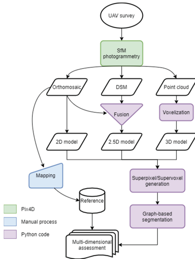
Figure 1. The methodology of the analysis followed for each landslide study site in the current study from raw data capture to segmentation and multi-dimensional assessment of UAV-derived models based on expert-based reference annotations. Each process is coloured by the software/technique used for the implementation while their products are mentioned in white frames.
