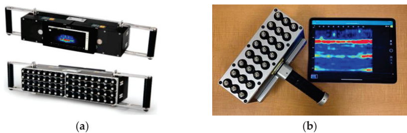
Figure 8. PAU systems used: (a) A1040 MIRA 3D (two devices were attached side by side to increase the number of channels to 16 rows of 4 transducers each) [115], (b) Pundit live array pro.
