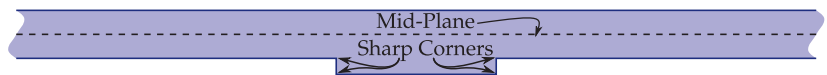
Figure 1. An exaggerated diagram showing a ‘hidden tamper’. The tamper is not symmetrically placed about the mid-plane and will therefore induce mode conversion between the two types of guided elastic waves.
