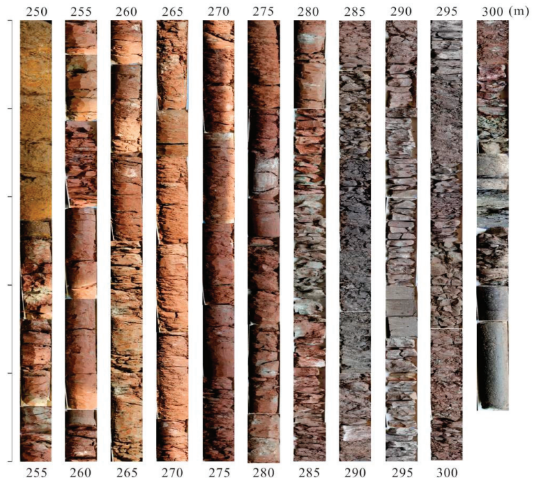
Figure 3. Lithology photos of the Pliocene strata in the core LQ11. Below 301 m, consists of a bedrock of black basalt; 301–252.7 m represents the Pliocene strata; and the lower stratum (301–283.5 m) is mostly dark red, while the upper section (283.5–252.7 m) is bright red, with the presence of calcareous nodules; above 252.7 m, consists of the Quaternary strata, yellow-brown coarse sand, and a mixture of gravel and clay.
