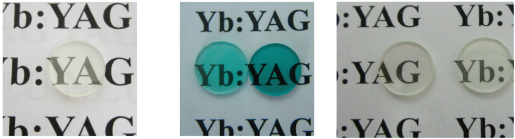
Figure 8. Photos of (\text{Y}_{1-x}\text{Yb}_x)\text{AG} transparent ceramics (1.2 mm thick), from left to right: x = 0, 0.01 and 0.1 , before annealing and x = 0, 0.01 and 0.1 , after annealing.
