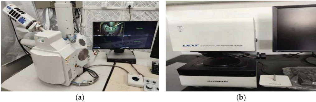
Figure 1. Macroscopic view of the main experimental instruments: (a) scanning electron microscope; (b) 3D confocal microscopy (LSCM).
