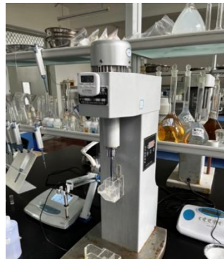
Figure 2. XFG flotation machine used for the flotation tests.
