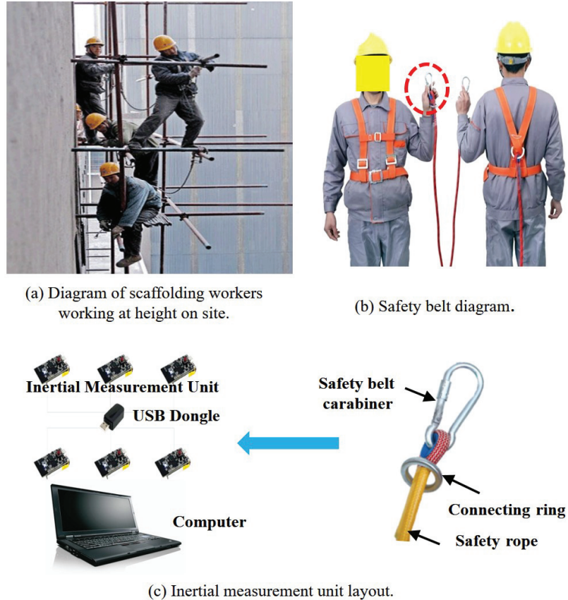
Figure 1. Schematic diagram of IMU-based scaffolding worker safety tethering action data acquisition.
