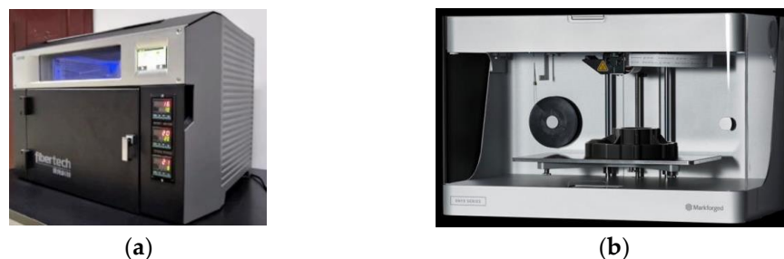
Figure 4. CFRTPCs-FDM printing equipment. (a) Combot-1™; (b) MarkTwo™.
