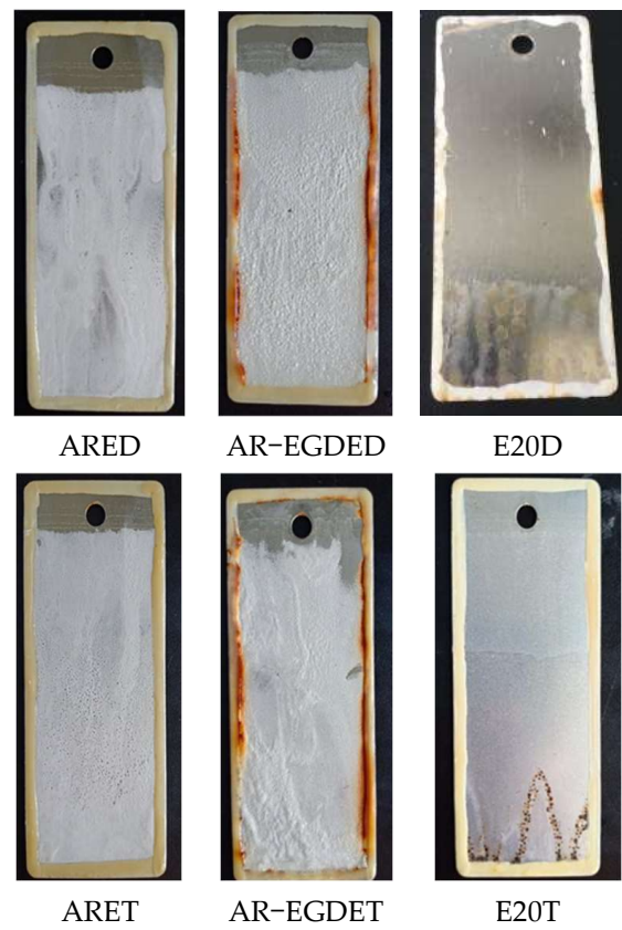
Figure 5. The images of immersion tests with water for 49 days.
