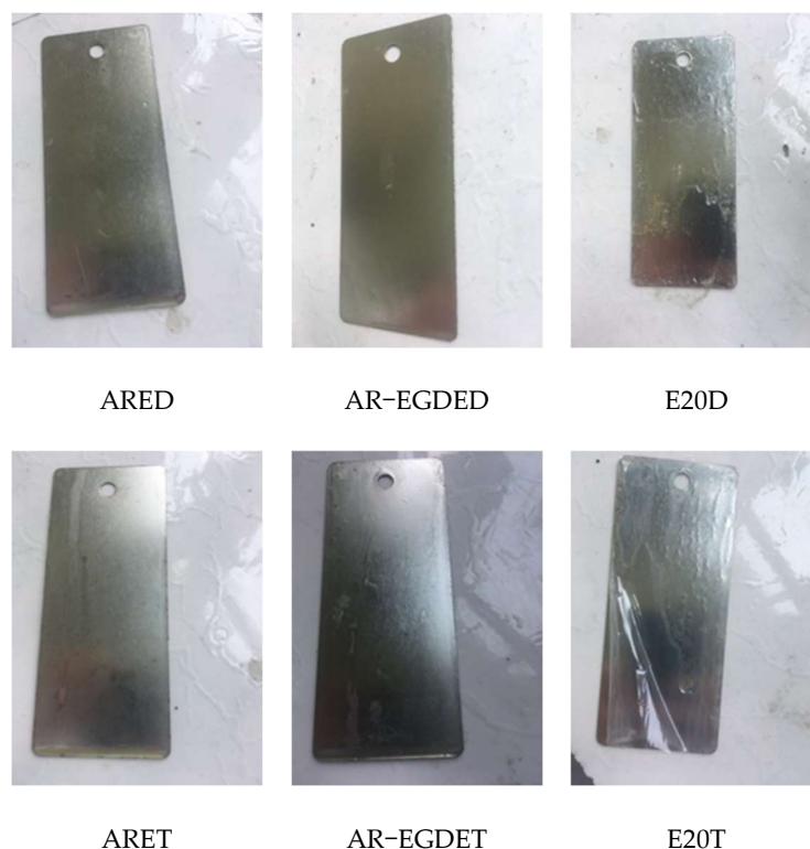
Figure 9. Photographs of the samples after the weatherability tests for 60 days.
