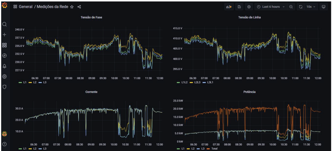
Figure 18. AC-Grid measurements for the solar power plant.
