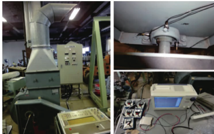
Figure 6. Rolling bearing failure test platform of Jiangnan University.
