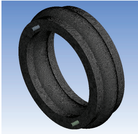
Figure 8. Bearing cavity grid.
