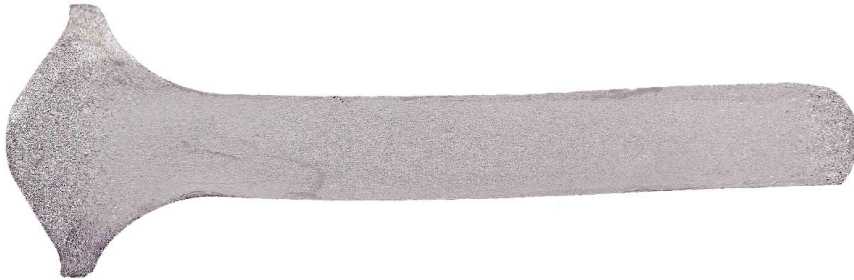
Figure 10. Macro structure of the analyzed sample obtained after macro-etching.
