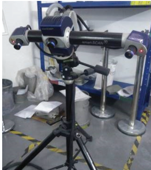
Figure 2. Breuckmann SmartSCAN3D scanner for the warpage measurements.
