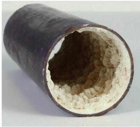
**Figure 1.** An example of a scale formed in a pipeline.
