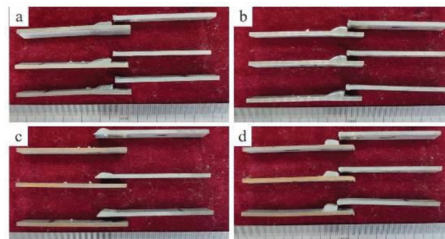
Figure 16. The fracture surface of the welded joints filled with different metals. (a) ER4043; (b) ER4047; (c) ER1070; (d) ER5356.
