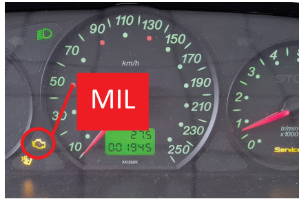
Figure 7. Photograph of gauges with malfunction indicator lamp on.
