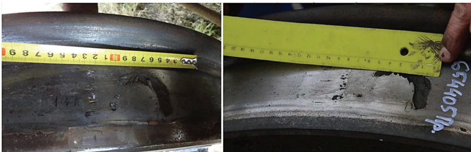
Figure 10. Two cracks in the wagon’s first wheelset wheel.
