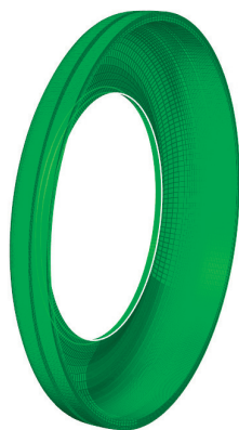
Figure 6. Half of the 3D finite element tyre model.
