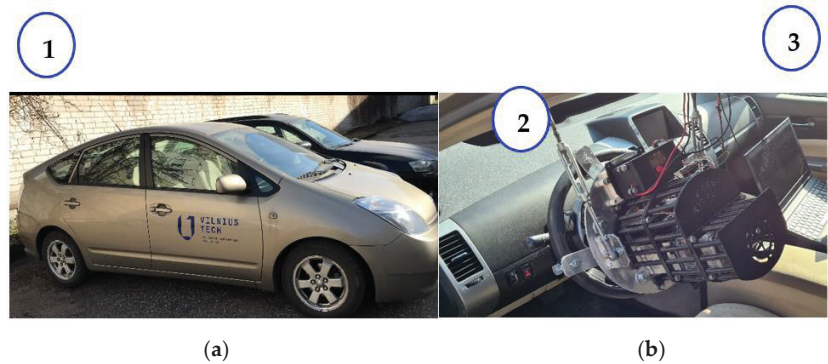
Figure 8. (a) The prototype of the first-level autonomous ground vehicle. (b) The automated steering device with the control computer.
