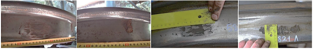
Figure 19. Wheel damage—flat and cracks.
