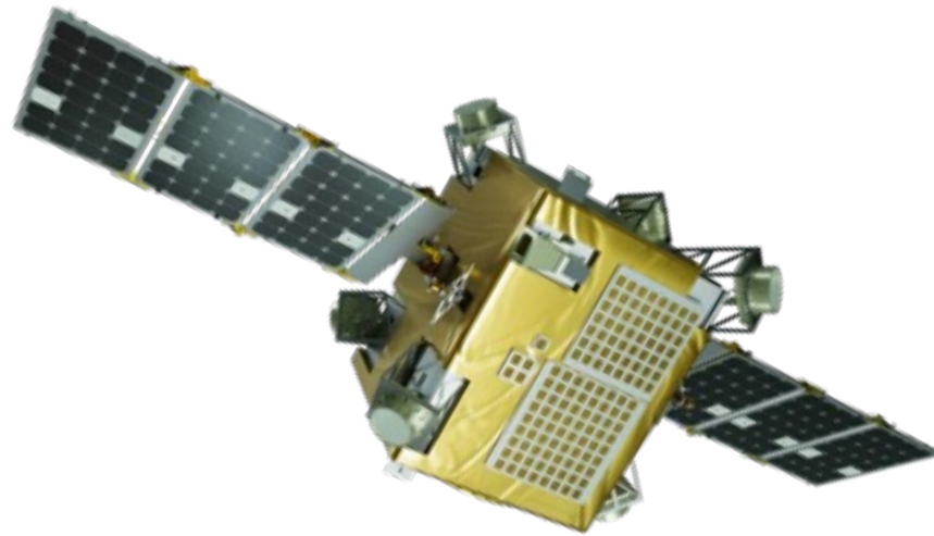
Figure 11. Six scintillating detectors positioned for an instantaneous all-sky field of view, no slewing required. Coupled with a cislunar orbit, MoonBEAM provides an unprecedented all-sky sensitivity that cannot be achieved in low-Earth orbit.
