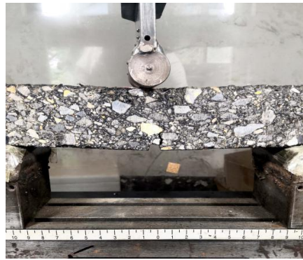
Figure 6. Bending failure of the beam specimen.
