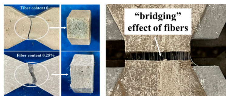
Figure 11. Tensile failure surface of fiber-reinforced solidified soil.
