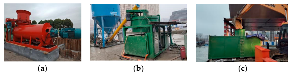
Figure 10. Equipment for the preparation and transportation of CLSM: (a) Soil metering device; (b) automated cement slurry preparation system; (c) intelligent CLSM mixing systems.
