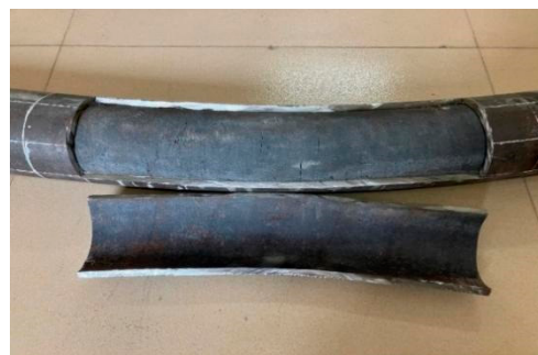
Figure 5. Typical damage pattern of the in-filled UHPC.
