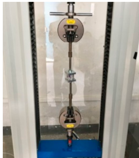
Figure 4. Bitumen bond strength (BBS) test.
