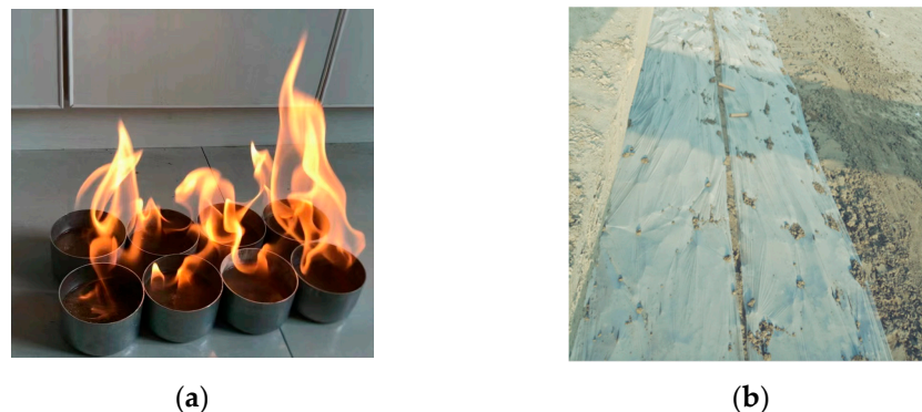
Figure 11. (a) Alcohol combustion method and (b) CLSM covered with plastic film.
