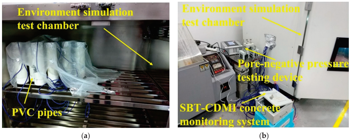
Figure 5. Concrete deformation and temperature monitoring test: (a) test molds and devices and (b) data receiving system.
