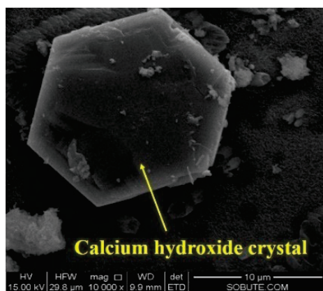
Figure 21. \text{Ca}(\text{OH})_2 with hexagonal plate structure formed by hydration of CaO expansive agent ( \times 10,000 ).
