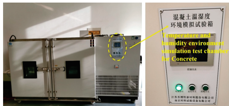
Figure 2. Temperature and humidity environment simulation test chamber for concrete.
