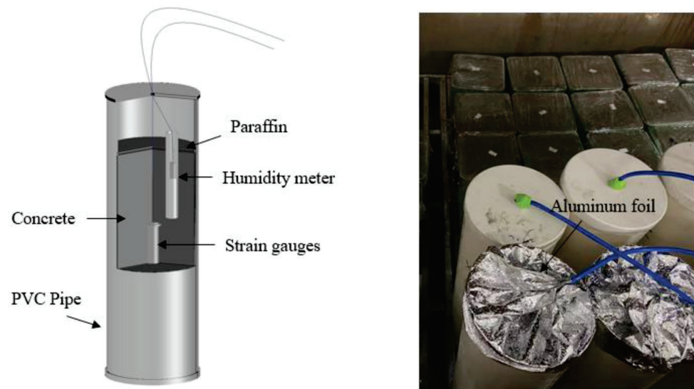
Figure 3. PVC pipe and PVC pipe in a variable temperature curing chamber.
