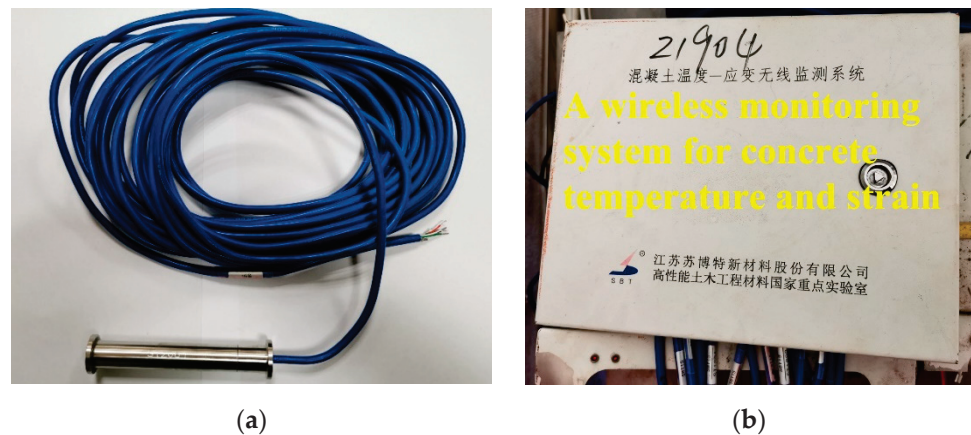
Figure 4. Monitoring by SBT-CDMI wireless monitoring system for concrete temperature and strain: (a) sensor and (b) data receiving system.
