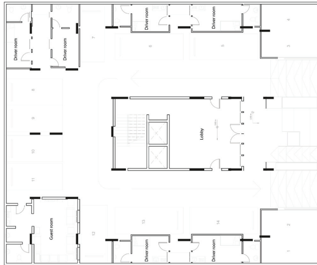
Figure 13. First floor plan (ground floor) (14 Parking spots, 6 Driver rooms, and 1 guest room).
