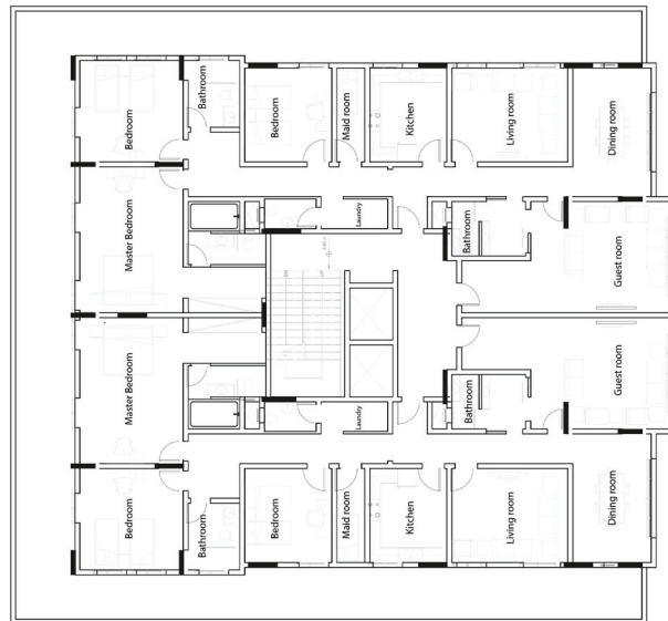
Figure 14. Repeated floor plan (3 bedrooms, 1 maid room, 1 kitchen, 1 living room, 3 bathrooms, 1 dining room, and 1 guest room).
