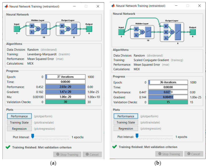
Figure 4. Training neural classifiers in the Deep Learning Toolbox of MATLAB: (a) feed-forward back-propagation ANN; (b) cascaded-forward back-propagation ANN.
