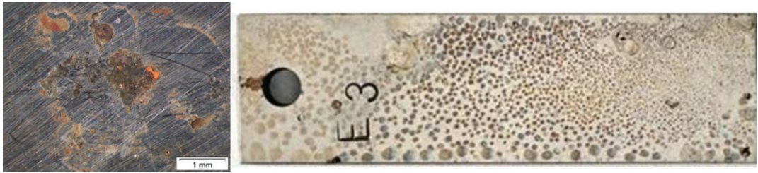
Figure 1. Left: SEM micrographs (8000 h at 60 °C/100 bar exposed to water-saturated supercritical CO 2 ) of the corrosion layer formed on X5CrNiCuNb16-4 with ellipsoidal peculiarity on hardened and tempered at 670 °C. Reprinted with permission from [16]. 2021 MDPI, A. Pfennig.
