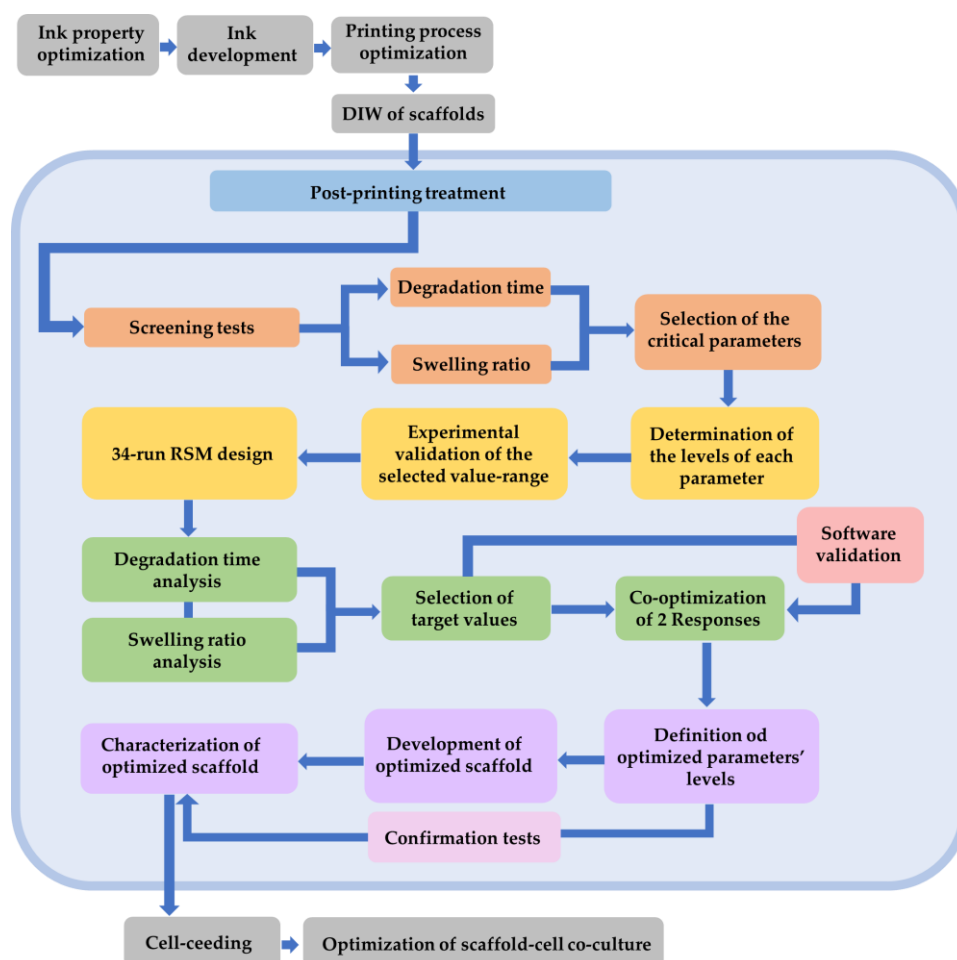
Figure 20. Flow diagram of the experimental procedure. The light blue area includes the main steps of this study.
