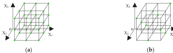
Figure 3. The method of sensitivity analysis: (a) full factor design; (b) orthogonal design.
