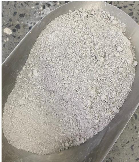
**Figure 4.** Metakaolin used for mortar preparation.
