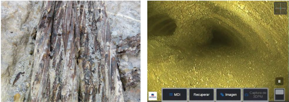
**Figure 10.** On the left, corroded cords and broken wires; on the right, unusual grout consistency with foam formation.
