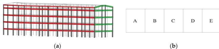
**Figure 1.** A schematic axonometric view of the FE model (a) and a plan view (b) of the building. A longitudinal and a transversal frame have been highlighted in the FE model (with beams shown in red and green colour, respectively). The letters in the plan view represent the different parts considered in the analyses, each one characterised at a given floor by constant mechanical properties of concrete and steel, as reported in Tables 1 and 2.
