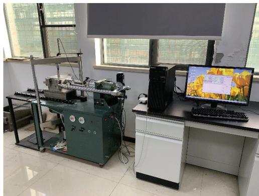
**Figure 1.** DZJ-1 large-scale direct shear test apparatus.
