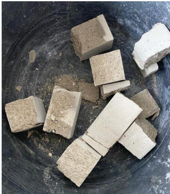
**Figure 6.** Crushed mortar samples prepared for leaching test.
