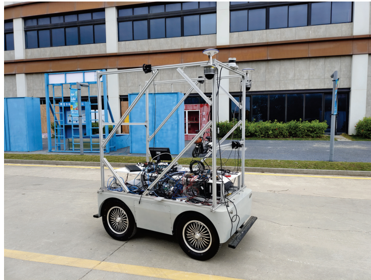
Figure 6. Illustration of our car equipped with the ouster-128 LiDAR and FDI integrated navigation system.
