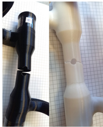
Figure 20. Post-test photograph of combined loading specimens (left specimen fabricated using Ultimaker© and right specimen fabricated using Fortus©).
