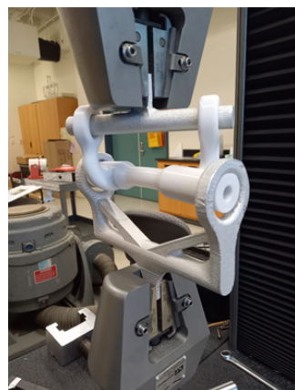
Figure 19. Combined loading specimen in the uniaxial test machine.
