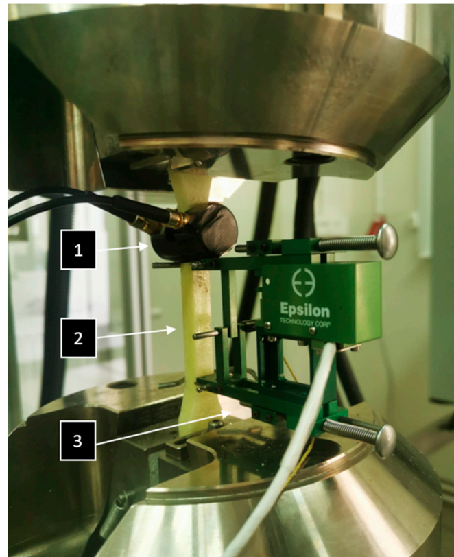
Figure 4. Specimen being tested (2) with an AE sensor (1) and an extensometer (3).
