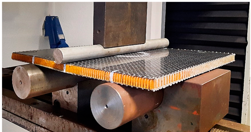
Figure 5. The experimental setup of the three-point bending tests.
