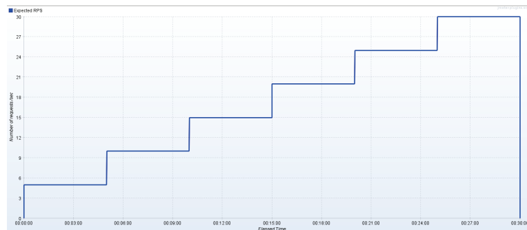
Figure 8. Step-wise increase in IoT data update load (with data integrity verification).
