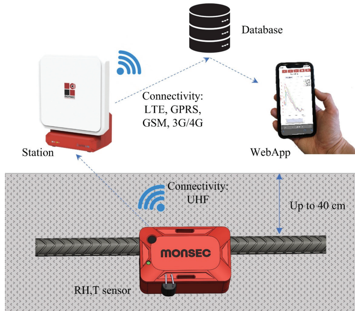
Figure 4. Components of the Monsec solution.
