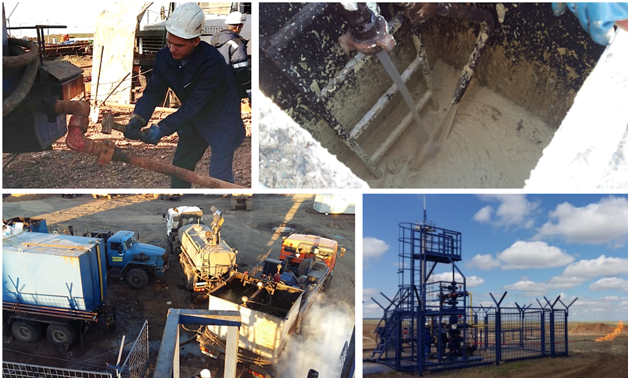
Figure 18. The process of preparing the blocking composition BHES-MC in field conditions, accompanied by pilot test and well discharge.
