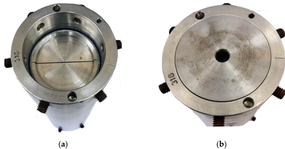
Figure 5. (a) Lower part of the filter press cell (exit point of the blocking composition from the crack); (b) Bottom plug of filter press (exit point of the blocking composition from the filter press).
