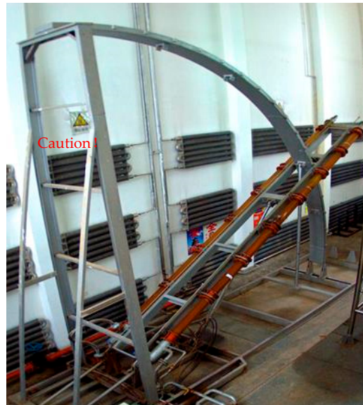
Figure 4. Photo of horizontal simulation well of Oil-water two-phase flow.
