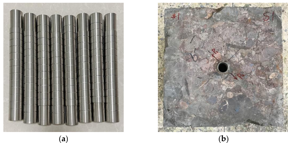
Figure 3. Wellbore and cementing. (a) Simulated wellbore made of steel; (b) rock samples after cementing.
