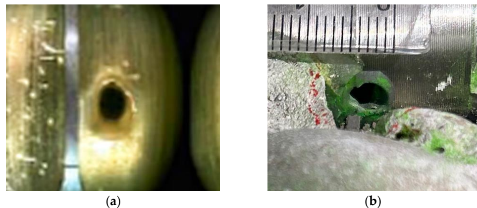
Figure 5. Perforation hole morphology. (a) The perforation hole took place underground in the field, showing an irregular circular hole; (b) the perforation hole made by the new water jetting apparatus, showing a similar morphology with the hole on site.
