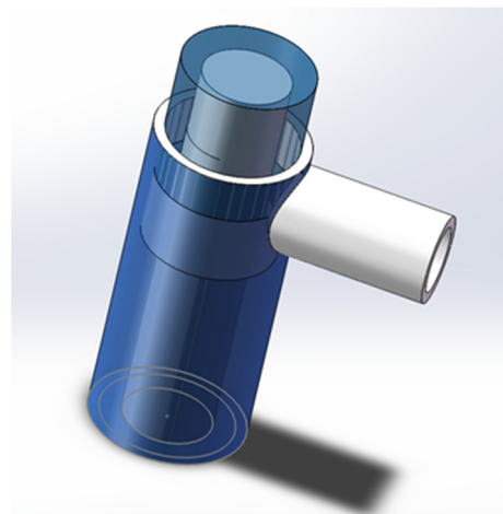
Figure 2. Schematic diagram of the structure of the choke valve.
