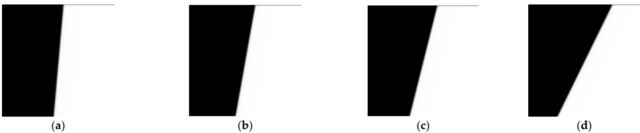
Figure 9. Images of slanted edge with different angles: (a) slanted-edge angle of 5°; (b) slanted-edge angle of 10°; (c) slanted-edge angle of 14°; (d) slanted-edge angle of 26°.
