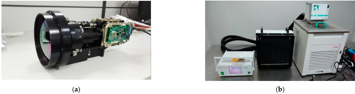
Figure 3. The infrared thermal imager and the blackbody source. (a) Infrared thermal imager; (b) Blackbody source.
