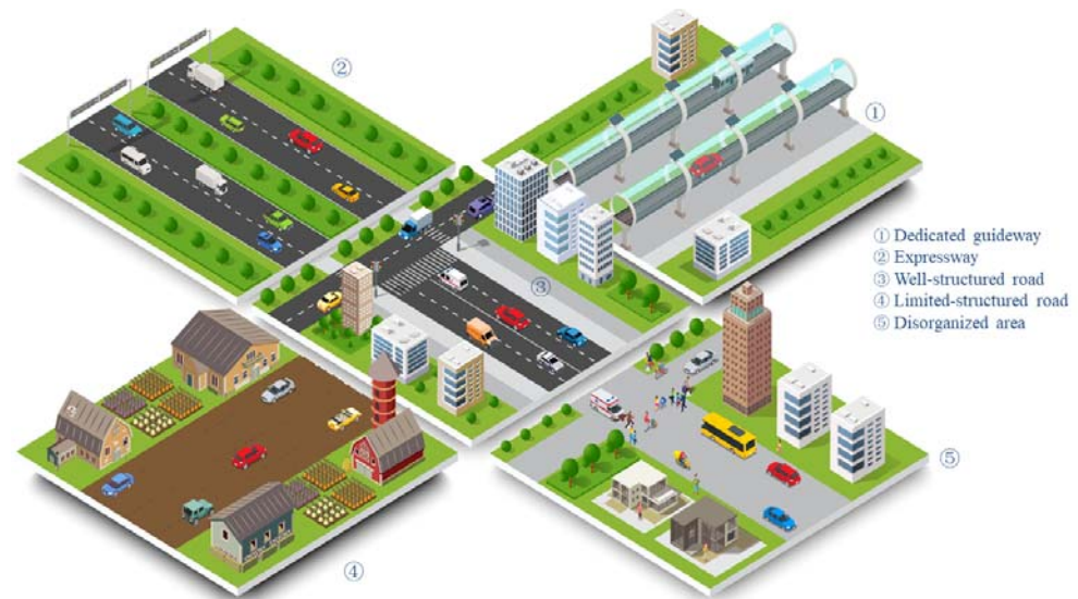
Figure 1. A bird’s-eye view of a simulated road network that comprises a variety of road types: dedicated guideways for AVs (labeled with ‘①’ at the top right), expressways (labeled with ‘②’ at the top left), well-structured roads (labeled with ‘③’ in the middle), limited-structured roads (labeled with ‘④’ at the bottom left), and disorganized areas (labeled with ‘⑤’ at the bottom right).
