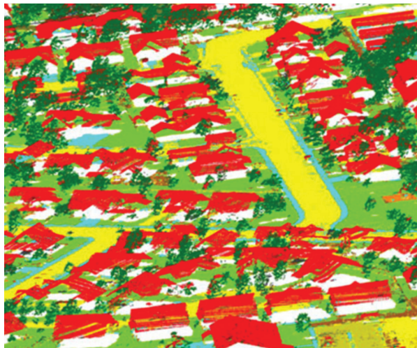
Figure 4. An example of a 3D point cloud classified into six classes (buildings, soil, grass, trees, asphalt, and concrete) by Ekhtari et al. [119].
