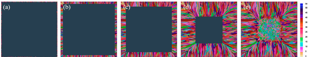
Figure 4. Superheat 60 K billet solidification process: (a) 1 s; (b) 42 s; (c) 92 s; (d) 202 s; (e) 252 s.
