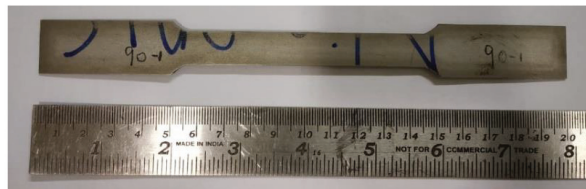
Figure 4. Tensile Test Specimen.
