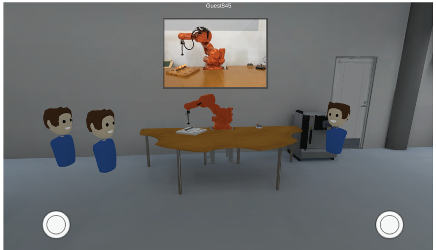
Figure 7. Multi-user XR robotic training session with a video stream of a physical robot.
