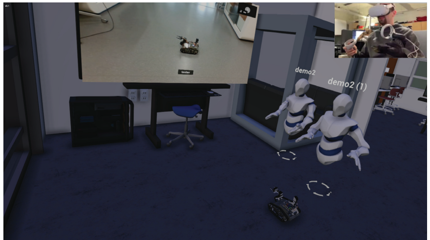
Figure 10. Visualization of the teleoperation of the robot, the video stream of the physical laboratory, the VR headset, and the smart gloves.
