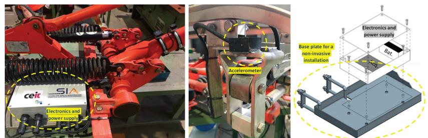
**Figure 12.** Installation of the monitoring system in the pantograph. Electronics and power supply (left); detail of an accelerometer (centre); detail of the base plate for a non-invasive installation (right).
