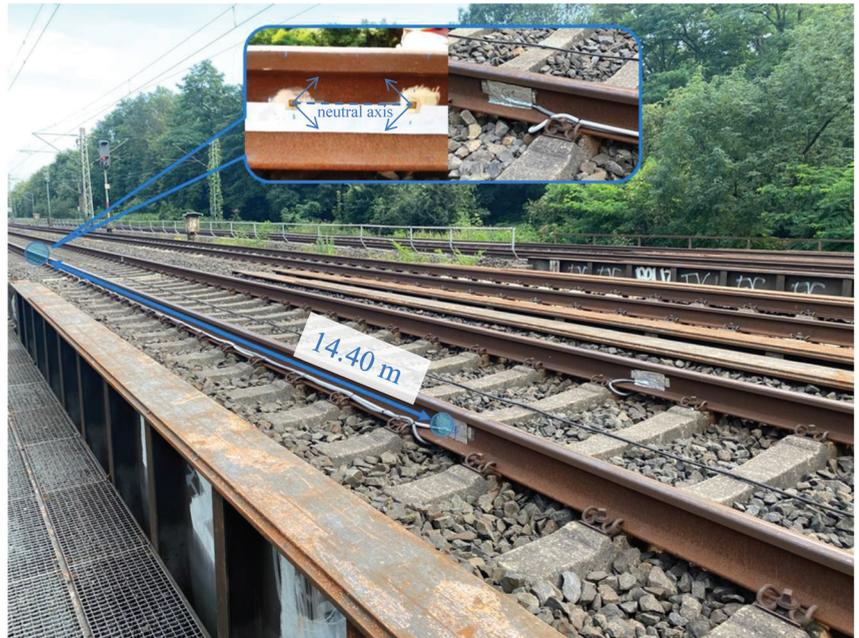
**Figure 4.** Top view of the bridge with the wheel load measuring points used at a distance of 14.4 m, with a detailed view of the rosette strain gauges and the weatherproof measuring point installed.
