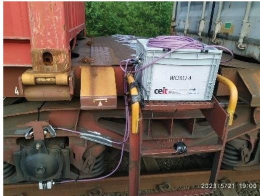
**Figure 15.** Installation of electronic components and antennas.
