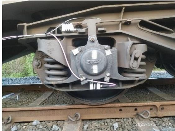
**Figure 10.** The arrangement of sensor nodes in the wagon.
