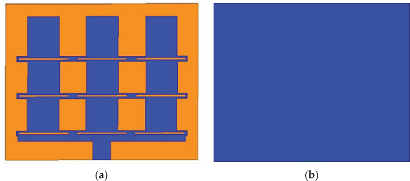
Figure 2. (a). Top view of the antenna (M) showing the patch array structure of the antenna, (b) bottom view of the antenna showing the full ground plane.
