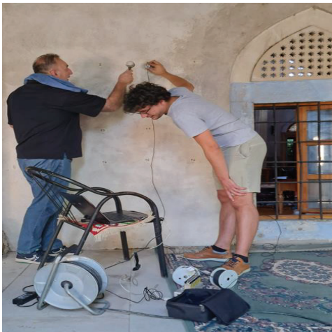
Figure 16. The emission of acoustic waves with a rubber hammer (outside) (author’s photo, 2022).
