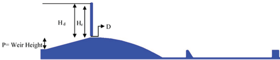
Figure 6. Operating conditions for gated/orifice flow.
