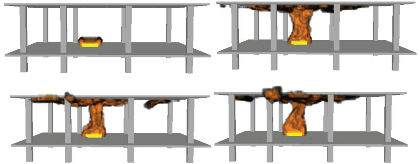
Figure 8. Flame shapes under the wind speed of 0 m/s.
