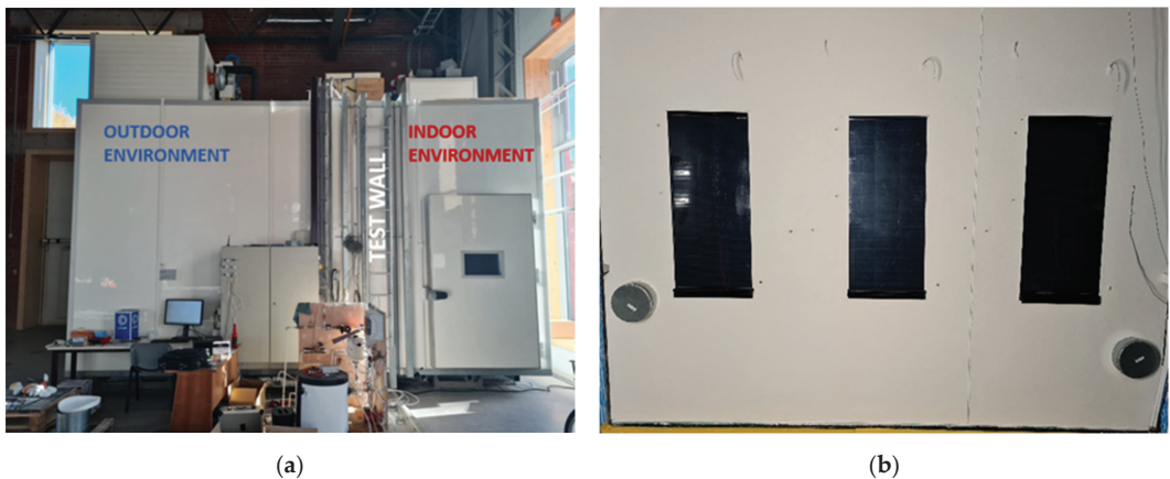
Figure 2. Climate chamber used for building the test wall (a) and the test wall inside the climate chamber (b).
