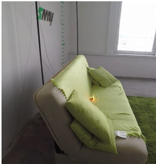
Figure 3. The location of the ignition source on the sofa at the beginning of a fire.
