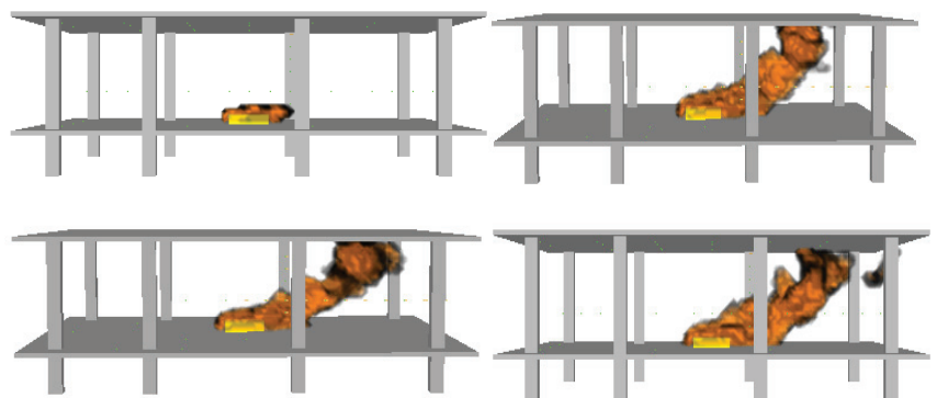
Figure 10. Flame shapes under the wind speed of 3 m/s.
