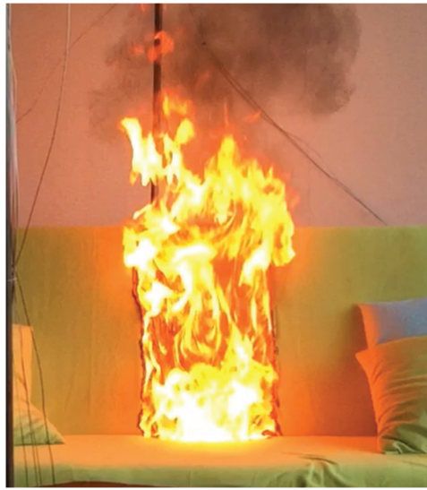
Figure 14. An image of u-shaped burning region (about 493 s of the first fire test).
