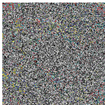
Figure 8. Ciphering process without a permutation process causes the circular structure of the iris to be recognizable.
