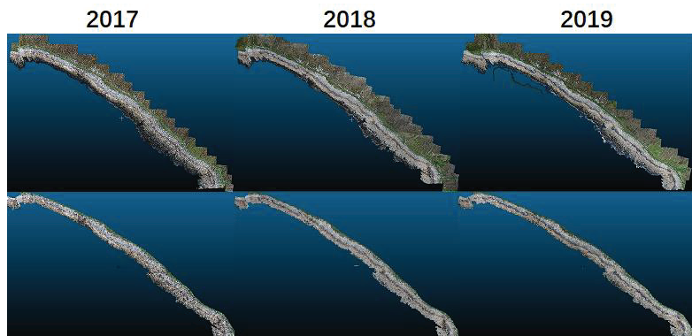
Figure 7. Point cloud models for the three-year span, where the top row shows the original clouds outputted by Pix4DMapper, and the bottom row indicates the clipped clouds.
