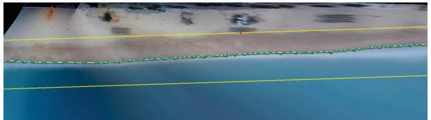
Figure 3. Example of shoreline extraction (green line) using a mask (yellow lines) to avoid features of the beach that might decrease the quality of the extraction. The background planview is in pixel coordinates.
