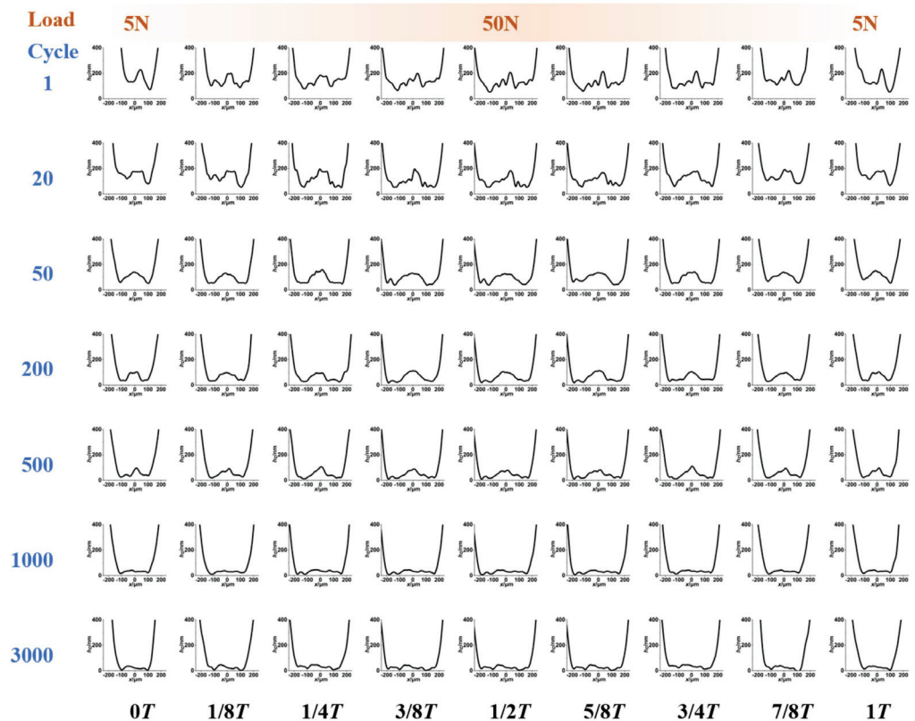
Figure 5. Mid-section film thickness distribution corresponding to Figure 4.
