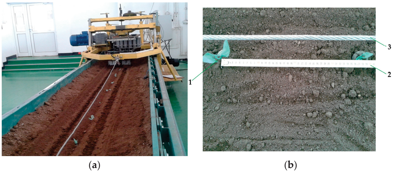
Figure 15. Seedlings simulacra in the soil bin: (a) planted in a row at the run end; (b) measuring the distance between seedlings: (1) planted seedling; (2) measuring tape; (3) towing cable.
