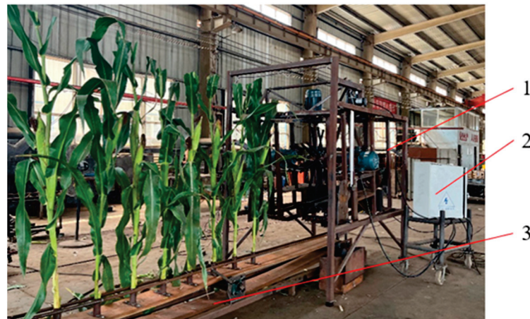
Figure 13. Physical image of the test bench. 1. Test bench. 2. Control box. 3. Feeding device.
