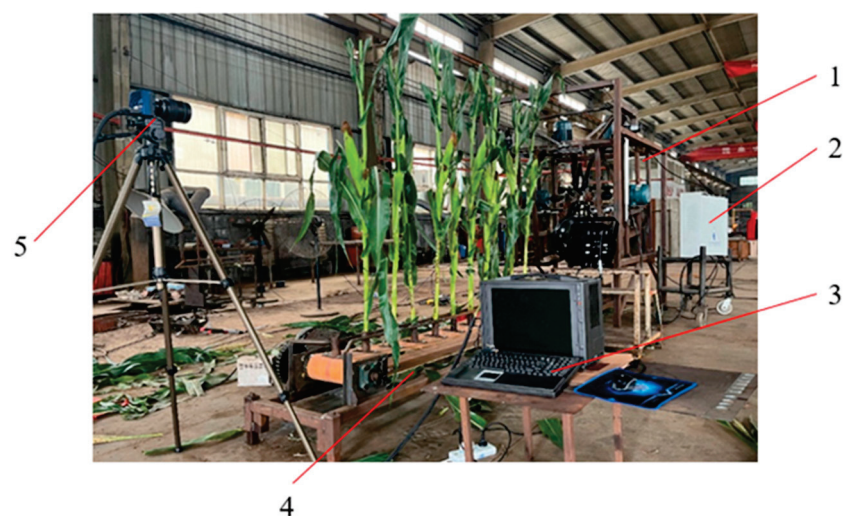
Figure 11. Image collection during ear-breaking process. 1. Test bench. 2. Control box. 3. Display. 4. Feeding device. 5. High-speed camera.
