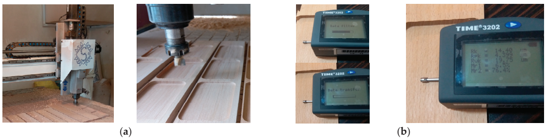
Figure 1. (a) CNC machining of beech wood; (b) surface roughness measurement.
