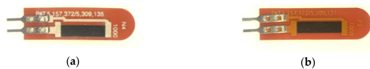
Figure 2. 1-inch bend resistive sensors: (a) polyester bend sensor and (b) polyimide bend sensor.
