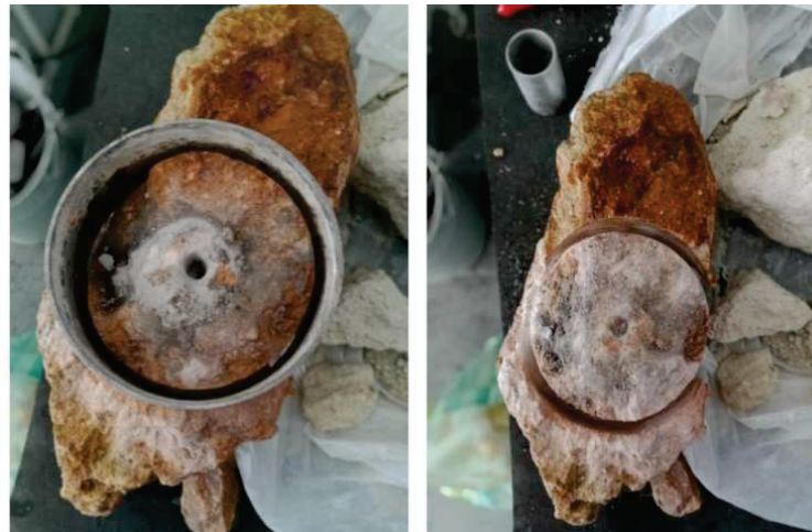
Figure 6. Rock sample from Hallaç Complex, which could not be cut to be used for impedance tube testing.
