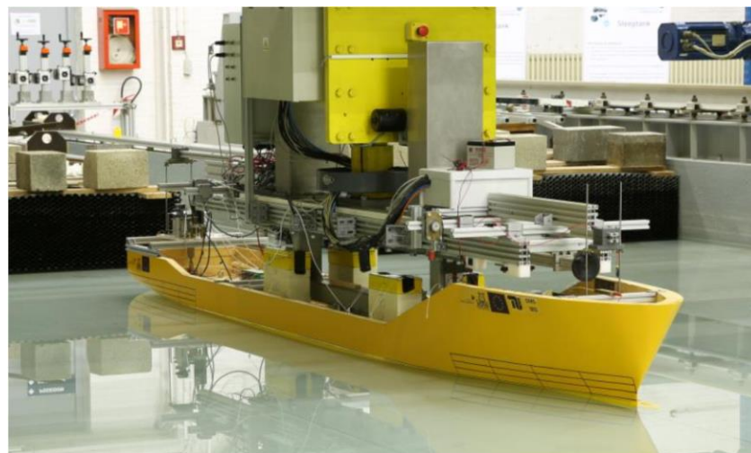
Figure 2. Planar motion mechanism tests of DTC ship model in shallow water. Reprinted from Ref. [63] with permission from Elsevier, 2023.
